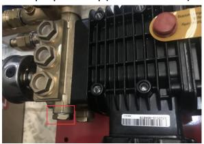
3. Connect 90DEG elbow (trottle control) together with pump's valve (red circled as below).
